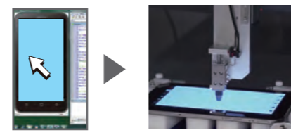
Robot operates the same place on the actual device when clicking on the virtual screen.
